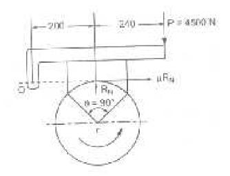
3. A 360 mm radius Brake drum contacts a single shoe as shown in figure (B2) and resists a torque of 250 Nm at 500 rpm. The co-efficient of friction is 0.3. determine
